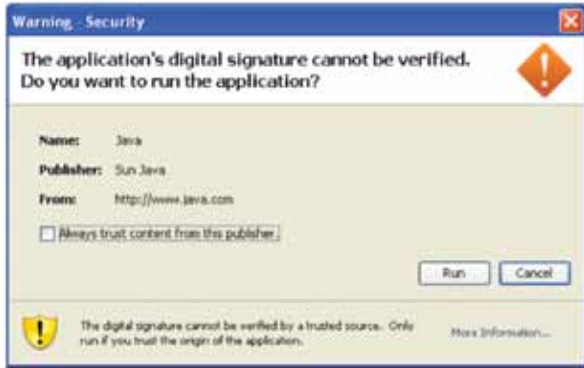
Figure 2. The Social-Engineer Toolkit can impersonate a Java applet and fool a victim into downloading malware.
