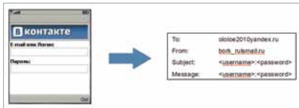
Figure 3. The phishing app J2ME/VkonPass.A steals login information and emails it to the attacker.
